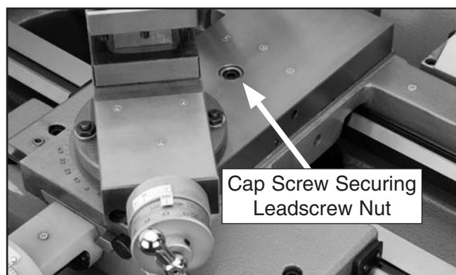
Figure 81. Location of cap screw that secures the leadscrew nut.
